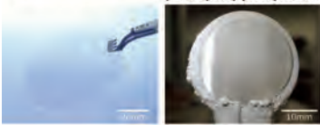
2-inch GaN crystal grown by the Na-flux method
