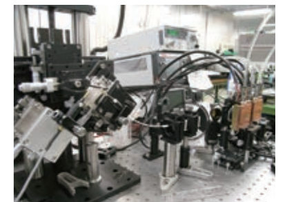
赤外光を用いた血糖測定器 Blood glucose measurement system using infrared light
