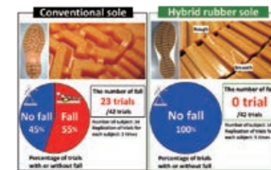
超耐滑靴底意匠の開発 Development of high slip resistant shoe outsole pattern
