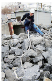
能動スコープカメラ Active Scope Camera Tested at a Fire Department
