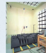
電波暗室(妨害電波耐性試験) Anechoic chamber (RF immunity test)
