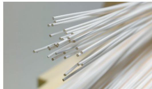
独自の熱誘起相分離法による強靱さと精密細孔を併せ持つPVDF中空糸膜 PVDF hollow fiber membranes featuring both toughness and a precise pore structure due to our unique thermally induced phase separation method
