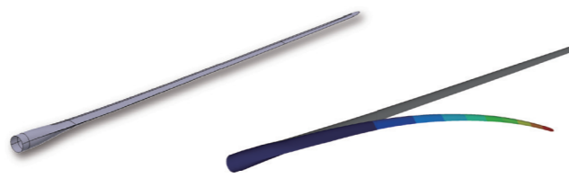
風力発電翼の解析例 構造モデル(左)、CAE解析結果(右) Example of wind power generation blade analysis; Structure model (left), FEA result (right)
